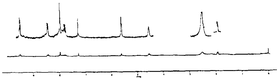
Figura 99.- Espectro de RMN- ^1\text{H} del complejo [(\text{CO})_2(\eta^2\text{-phen})\text{Mo}(\mu\text{-Cl})(\mu\text{-CO})\text{Rh}(\text{COD})] .
