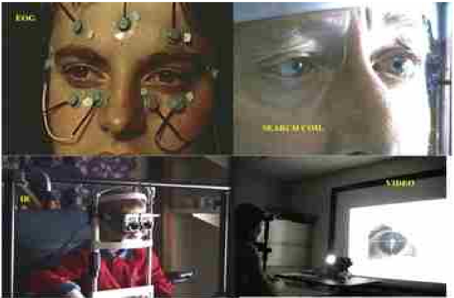
Figure 4 (Hertle): Eye Movement Recording Techniques. The four most common recording techniques (electro-oculogram EOG, infrared reflection devices IR, scleral search coil, and video-oculography, VOG) vary according to spatial and temporal resolution, capability to record multiple degrees of eye freedom, setup complexity, system specific artifacts, and invasiveness.
