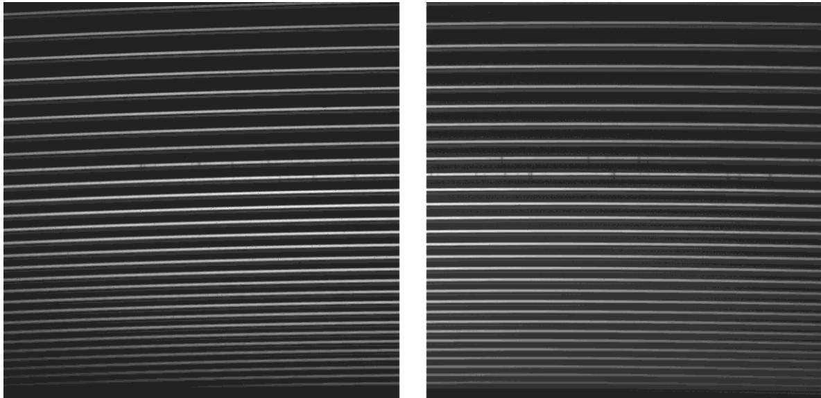
Figure 10. Spectrum taken on CARMENES-NIR produced by flat illumination (CVC-5).
