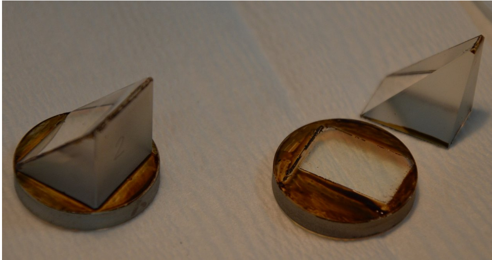
Figure 6.: The image slicer broken after transport.: The dark surface had been treated with sealing paint which most probably caused the loss of optical contact due to high temperatures during transport..
