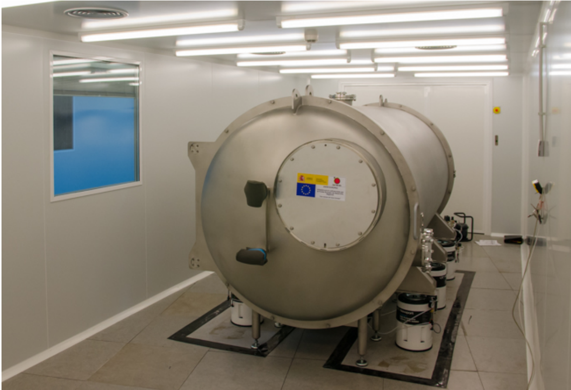
FIGURE 1.6— Visible vacuum tank inside the thermal controlled chamber at the coudé room of the Calar Alto 3.5 m telescope.
