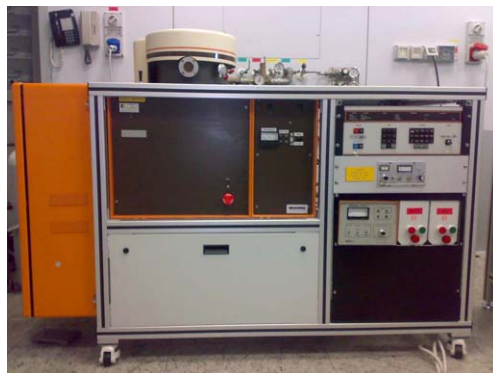
Figure 3-3. Photograph of an Oxford Reactive Ion Etcher
