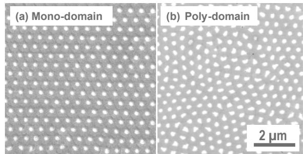
Fig 1: Scanning electron micrographs of nickel filled alumina templates fabricated via imprint lithography (a) and using two steps anodisation process (b).
