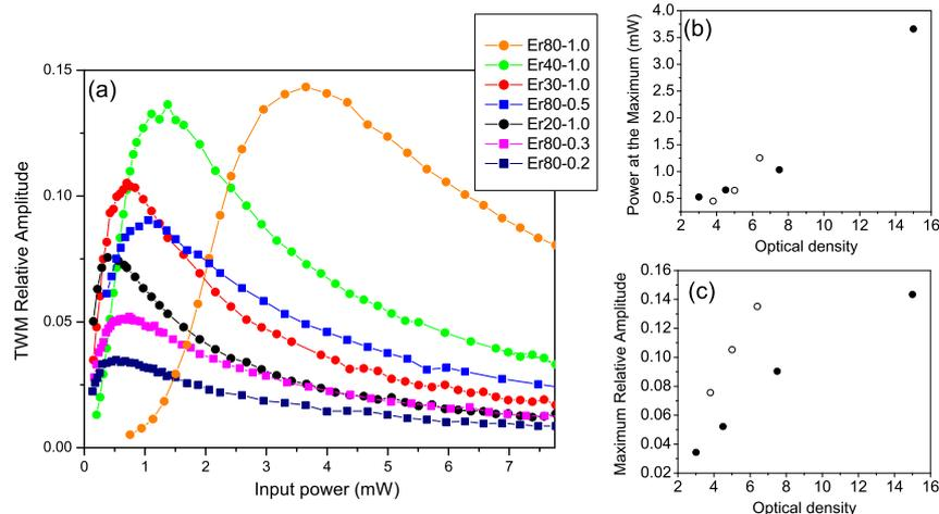
**Figure 1:** (a) TWM relative amplitude as a function of input power for fibers with different ion concentration. Maximum relative amplitude (c) and power at that maximum (b) as a function of optical density. For (b) and (c): Moderate doped fibers (open circles); highly doped fibers with ion concentration of 3150 ppp (closed circles).
