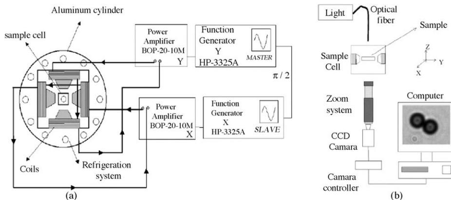
Fig. 1. Experimental setup used to (a) generate the magnetic fields in the plane of the sample ( $X - Y$ ) and (b) to record the images.
