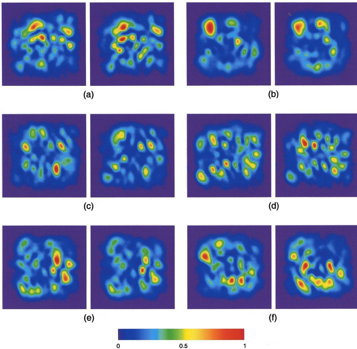
FIG. 2 (color online). Six representative pairs of instantaneous consecutive patterns separated by a time delay  $t_d = 0.6$  ns. The transmitted pattern (left) is recorded a time  $t_d$  before than the reflected pattern (right). Experimental pattern dimension  $20 \times 20$  mm.
