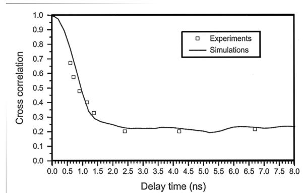
FIG. 4. The maximum value of the cross correlation function between consecutive patterns versus the time delay  $t_d$ . Each point corresponds to an average over approximately 200 laser pulses. The solid curve corresponds to the numerical simulations.
