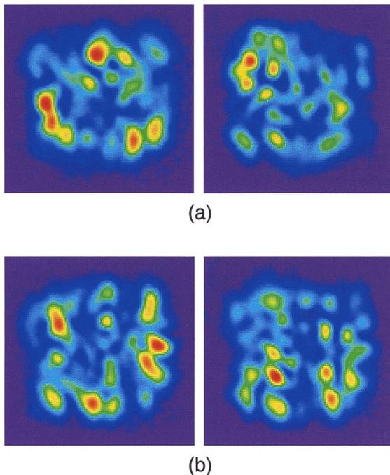
FIG. 3 (color online). Representative pairs of consecutive instantaneous patterns separated by a time delay of (a)  $t_d = 4.3$  ns and (b)  $t_d = 6.8$  ns. The transmitted pattern (left) is recorded a time  $t_d$  before than the reflected pattern (right). Experimental pattern dimension  $20 \times 20$  mm. The color scale is the same as in Fig. 2.
