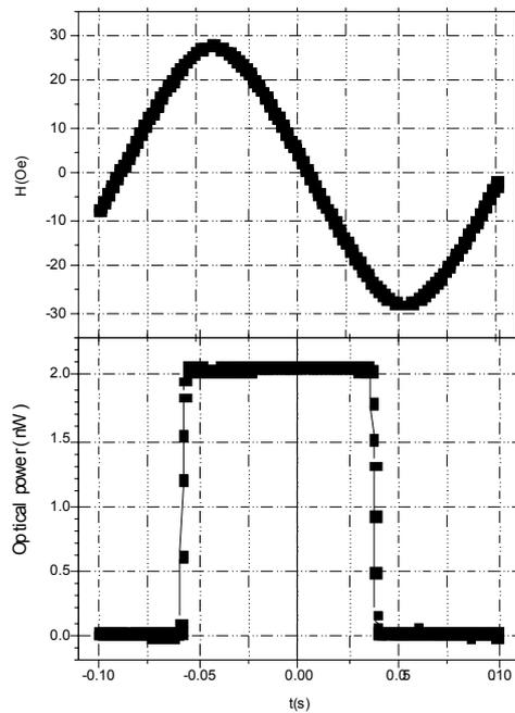
**Figure 2:** Applied field and variation of the diffracted light at an angular position corresponding to the stripe array periodicity when light is shined from the flat side of the structure.
