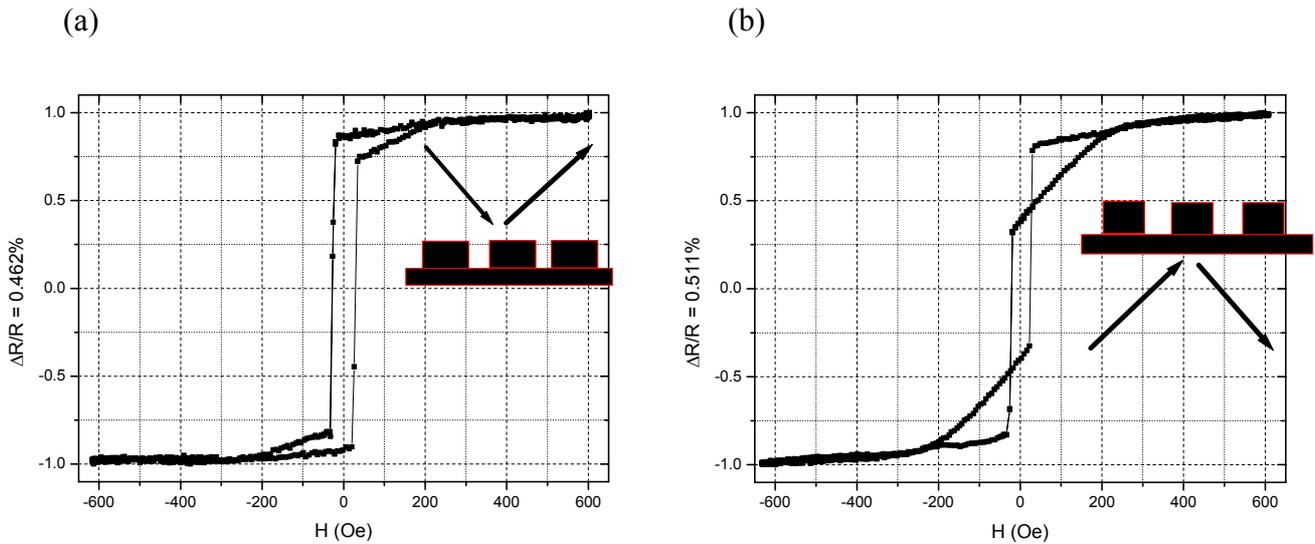
**Figure 1:** Hysteresis loops for a structure consisting of a continuous Co film with an array of Co stripes on top when the light is shined from (a) the patterned side, and (b) the flat side. The insets show the magneto optical measurement configuration (see text)
